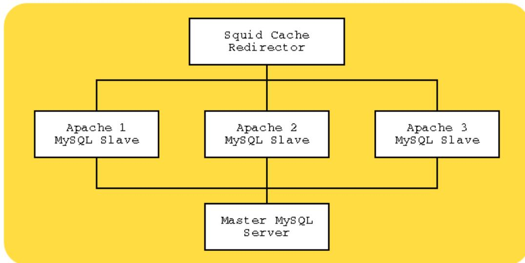
You would then write your application to send all database writes to the master server and all reads to the local slave. It is also possible to set up two-way replication, but you would need to supply your own application-level logic to maintain atomicity of distributed writes. And you lose a lot of the advantages of this architecture if you do this as the writes would have to go to all the slaves anyway.
